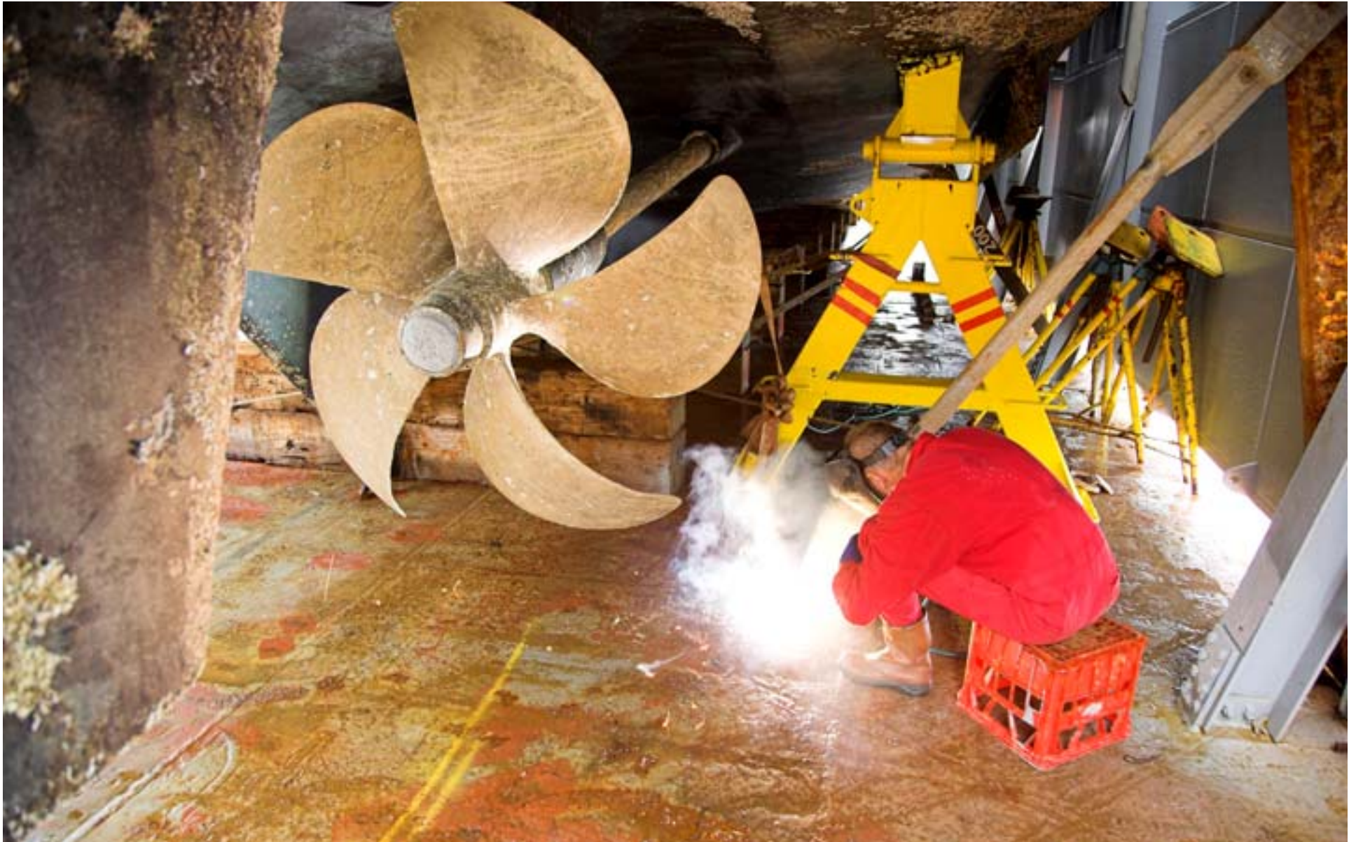
18. These sea fastenings are welded to the deck of the vessel and tensioned to the hull of the yacht. This is a time and energy consuming process.
